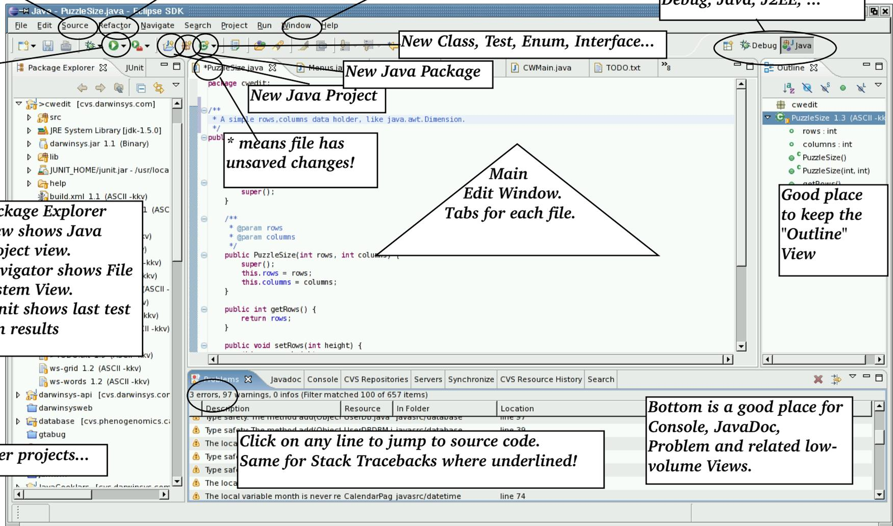
**Shortcuts:** CTRL/L go to line #; Alt/Shift/R Rename; CTRL/Shift/R Open Resource (file) by name; Alt/Shift/I Inline, Alt/Shift/M Extract Method, Alt/Shift/L Extract Local Variable; CTRL/Shift/F Format code; CTRL/Shift/P goto matching Paren; CTRL/Shift/O Organize Imports, many more...
